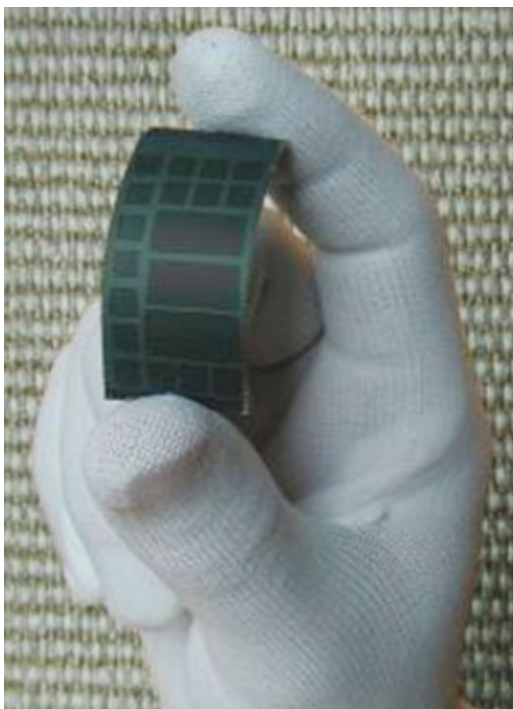
Figure 8 Illustration of the flexibility of PV cells on glass-fiber fabric. [Color figure can be viewed in the online issue, which is available at www.interscience.wiley.com .]
